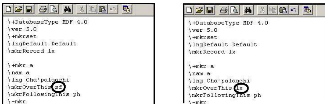
Figure 1.5. Example: Redefining the position of the marker in the .typ structure file. Before: defined under 'sf'. After: defined under 'lx'
